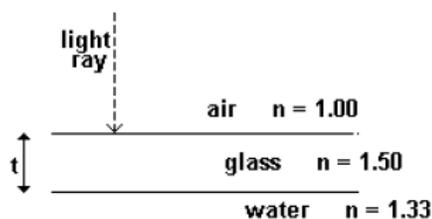
A light ray is incident normal to a thin layer of glass. Given the figure, what is the minimum thickness of the glass that gives the reflected light an orangish color ( $\lambda(\text{air})$  orange light = 600nm)
