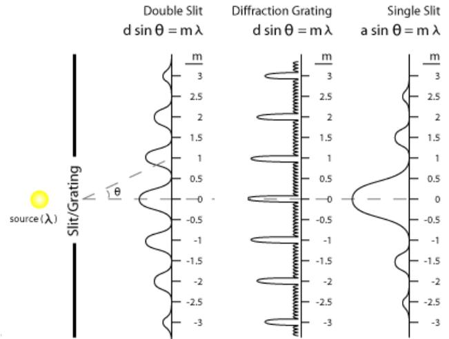
In Young's double slit experiment, the second order bright band of one light source overlaps the third order band of another light source. If the first light source has a wavelength of 660 nm, what is the wavelength of the second light source?
